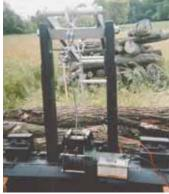
Grapple fork is opened and closed by a rocker arm mounted between two uprights.
