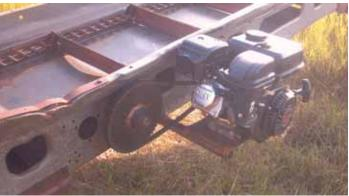
Craig Spierling replaced the pto drive on his bale elevator with a gas engine, eliminating the need for a tractor.
