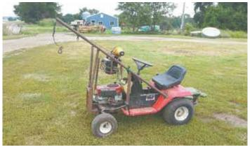
Cody Powell converted his MTD riding mower into a garden tractor "tow truck". An electric winch mounts in front of the steering wheel within reach of the driver.
