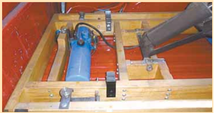
There wasn't room under the pickup bed to mount a hoist and hydraulic pump, so he built a unit that slides into the S-10 box.
