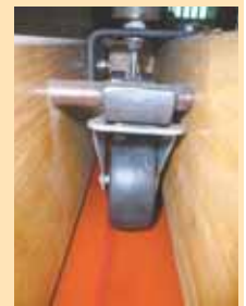
Lower frame supports the hydraulic hoist and has brackets for the rear pivot point. Four retractable wheels are used to roll the box in and out.
