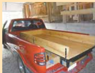
Double wall subframe spreads the weight across the entire pickup box. The upper frame supports the floor and sides of the dump box, which extends beyond the bumper.
