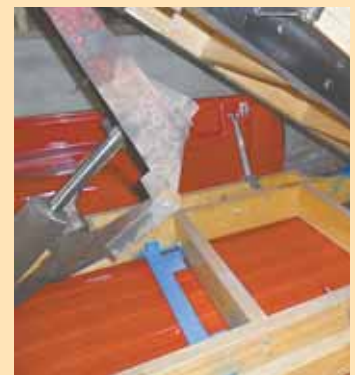
Double wall subframe spreads the weight across the entire pickup box. The upper frame supports the floor and sides of the dump box, which extends beyond the bumper.
