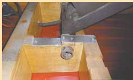
Lower frame supports the hydraulic hoist and has brackets for the rear pivot point. Four retractable wheels are used to roll the box in and out.
