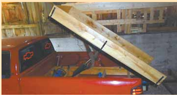
Jerry Maddock turned his Chevy S-10 pickup into a mini dump truck equipped with a rollaway dump bed.
