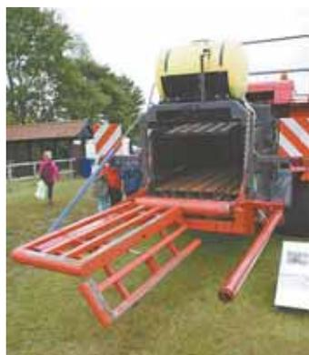
Big square baler-mounted tray automatically sets bale on edge in the field for easier lifting and loading.
