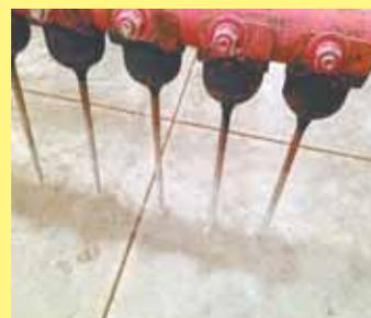
Rake is equipped with a series of rubber-mounted teeth.
