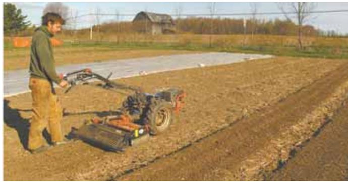
Jean-Martin Fortier makes a good living on a tiny farm using only hand tools and this BCS walk-behind tractor, shown here pulling a rotary-powered harrow.
