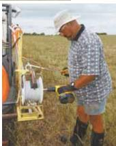
Polybraid wire reel holder mounts on front of an ATV or utility vehicle and is operated by a cordless drill.
