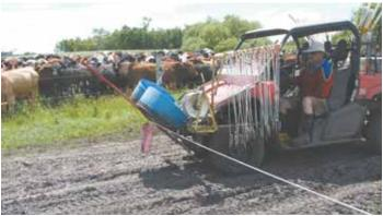
Neil Dennis's fence crosser mounts on front of his utility vehicle at an angle, allowing him to drive right over a fence wire and bypass gates. Note wire reel holder and adjust-
