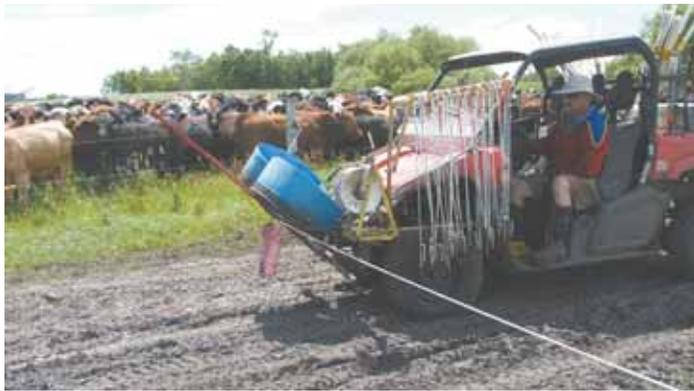
Neil Dennis's fence crosser mounts on front of his utility vehicle at an angle, allowing him to drive right over a fence wire and bypass gates. Note wire reel holder and adjustable pigtail post holder.
