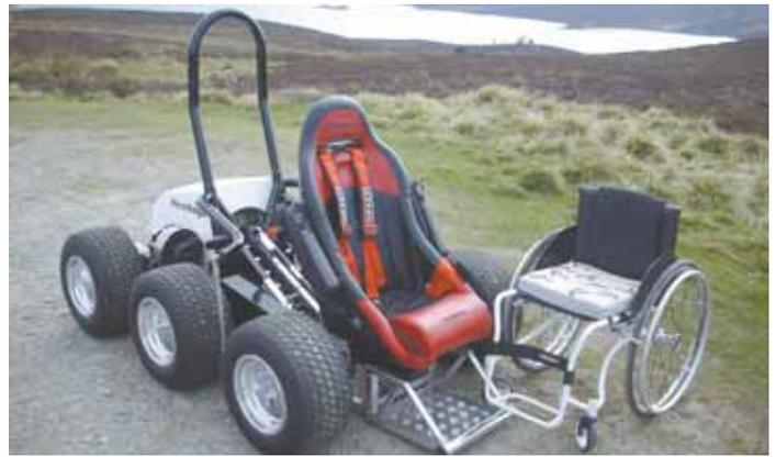
Front-mounted seat on the 6-WD HexHog is designed to make transfer from a wheelchair easier. The transfer mechanism lowers the seat and extends it out ahead of the front wheels.
