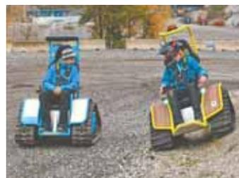
Powered by a modular lithium ion battery system, new all-terrain tracked chair moves easily over nearly all surfaces.
