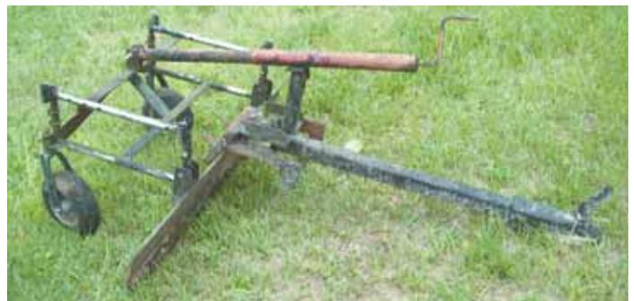
Hand crank attached to wheelchair frame is used to raise and lower grader's 42-in. blade.
