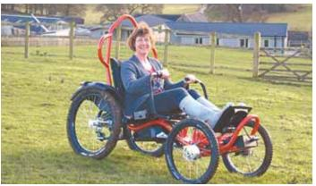
Off-road wheelchair comes with handlebar control, including a twist grip throttle to accelerate and fail-safe braking. Joystick control is also available.
