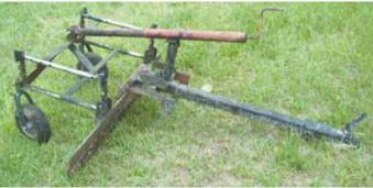
Hand crank attached to wheelchair frame is used to raise and lower grader's 42-in. blade.
