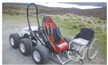
Front-mounted seat on the 6-WD HexHog is designed to make transfer from a wheelchair easier. The transfer mechanism lowers the seat and extends it out ahead of the front wheels.
