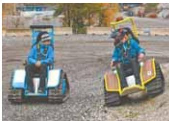
Powered by a modular lithium ion battery system, new all-terrain tracked chair moves easily over nearly all surfaces.
