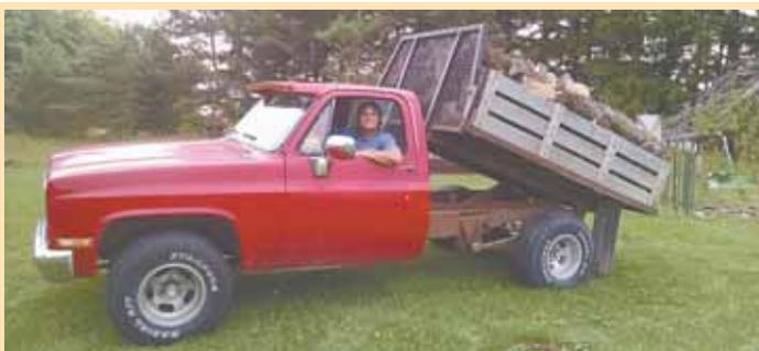
Craig Spierling mounted a 1 1/2-yard dump box on his 1980 Chevy pickup. Originally the pump was driveshaft-driven, but he modified it to run off a 1/2-in. electric drill.
