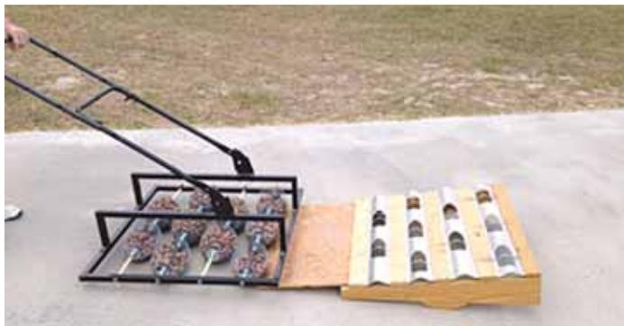
Rolling nut gatherer is filled with 10 wire baskets mounted on a steel frame to pick nuts up off the ground.
