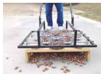
Baskets match up with corresponding holes cut into unloading rack.
