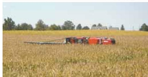
Cover crop seeding system is designed to fit the Dahmers' Miller Nitro 5240 high clearance sprayer. Photo at left shows cereal rye being seeded into standing corn.
