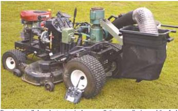
Remote-controlled, garden tractor-sized mower pelletizes grass clippings and then feeds the pellets into a burner that powers the machine.
