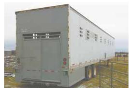
Gary Bueckert saved the cost of a new cattle hauler by converting a semi trailer into this ground loading model. The former 53-ft. van carries about 30 head at a time.
