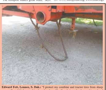
corn stalk stubble by attaching lengths of no. 60 roller chain under the machines ahead of each row. On the combine, I leave enough slack so that when the header is down, the chain hangs on the ground in a U-shape. As it drags along, the heavy chain bends stalks forward and away from the tires."
