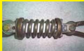
wire as it is stretched. The tension is calibrated in kilonewtons (Kn) – from 0 to 2.5 Kn. It lets you build fence that is consistently tight. I have had this tool for over 20 years and now have need for another one. It was made under the Allflex name and was probably made in New Zealand, but no one at Allflex recognizes it. I've done a lot of searching
