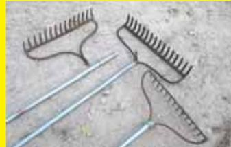
missing handles. I made new ones out of electrical conduit that I had laying around the place. I cut off half the pipe about 4 in. up from one end to form a tab. Then I slipped the rake head into the pipe and folded the tab back down against the pipe to hold the rake head in place. A band clamp holds it in place. Now I've got a pile of rakes I can use again or give away as gifts. **(E.D. Kramer, bruland@yahoo.com)**
