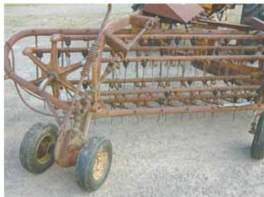
Allen Kimball converted an old 3-pt. mounted, pto-driven rake into a pull-type, ground-driven unit.
