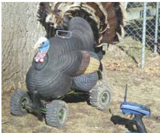
Remote-controlled robotic turkey has a wide stance and low center of gravity.
