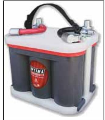
Custom CNC-machined battery pack includes a pair of Optima 6-volt AGM Red Top batteries harnessed together in parallel. They provide 2,000 cranking amps of 6-volt power.
