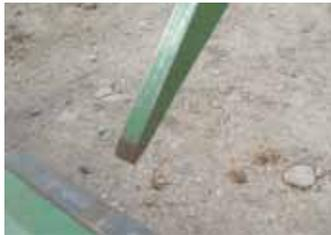
**Grapple tooth sharpened by Gutschmidt.** most of the problems could be avoided by sharpening the grapple fork teeth. When grapples come from the factory, the teeth are usually pretty blunt. It takes a lot of hydraulic force to push the tines into dense bales, putting stress on the arms and tines
