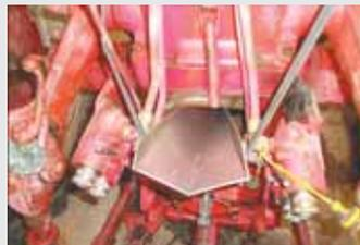
**After the rebuilt pto unit has been bolted back onto tractor, Grenzow uses this homemade trough to refill with oil.**
