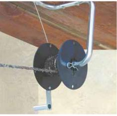
Reel-to-reel system stretches 1/4-in. glue tape about 6 in. below the ceiling. Once the tape is full of flies you crank it up to expose fresh tape at the other end.
