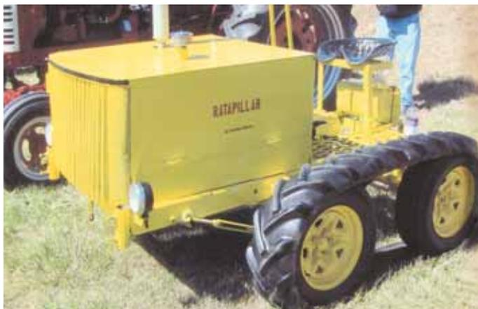
Layman Cornelison's "Ratapillar" is powered by a 1980 Chevette engine. Tracks were made from the rear tires off a Farmall C tractor.
