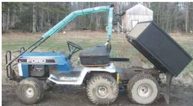
James Batchelder converted his 1980's Ford 16 hp. garden tractor into this 4-WD, tandem axle model equipped with a dump box.
