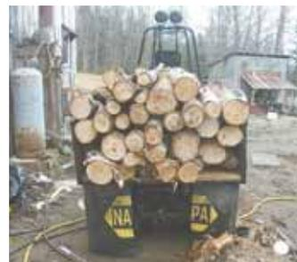
He uses a hand-operated boat winch to operate the dump box, which has a capacity of about 1,200 lbs.
