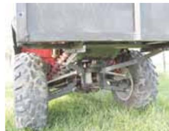
Bottom of box pins to 4-wheeler's receiver hitch.
