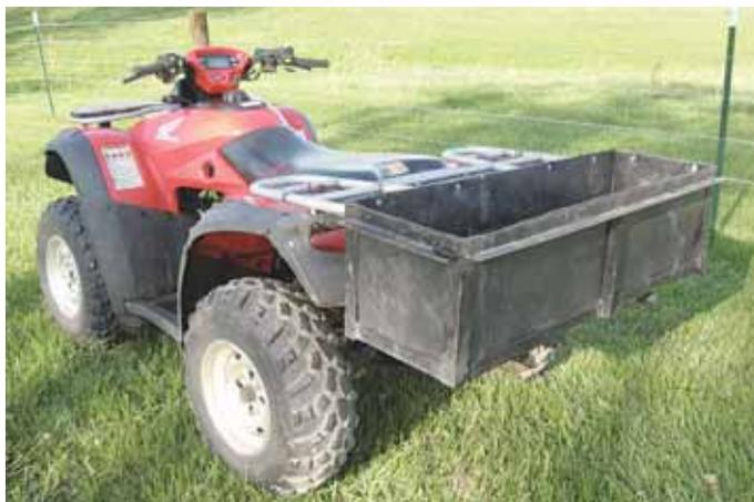
Cargo box is designed to reduce overhang stress on 4-wheeler and results in minimum "squatting" when hauling a heavy load.
