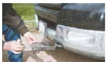
Hitch slips over pickup's tow hook. A steel pin inserts from underneath through the tow hook.
