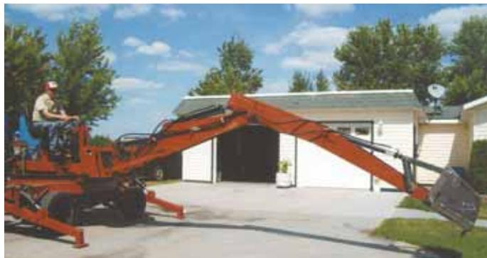
A hydraulic pump belt-drives a pair of tubeless rubber wheels that ride inside around top of turntable. Bucket can reach out 16 ft. and down more than 10 ft.
