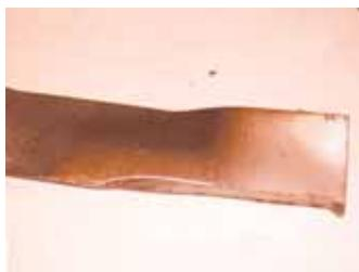
Unsharpened "finger" at end of blade knocks stones out of the way and acts like a hook to pull grass into blade.
