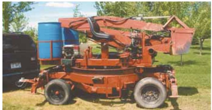
Self-propelled excavator is mounted on a powered 6-ft. dia. turntable that supports the boom. A pair of 55-gal. barrels on back are filled with water to serve as counterweights.
