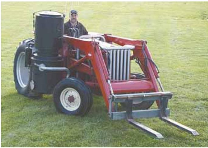
Ron Lemler's wood gas-powered tractor runs on wood scraps from his pallet factory.
