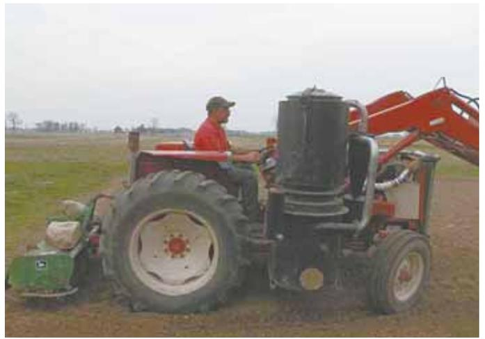
Last spring the 1978 IH 574 tractor powered a 4-ft. tiller.
