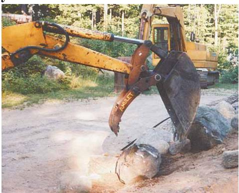
Hoe Clamp moves as bucket moves. Lund says it's easier to use than a "hydraulic thumb".
