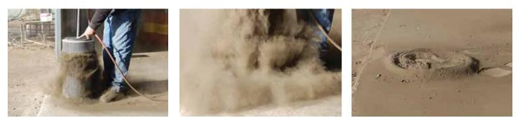
During tests on a pair of Deere 7750 tractors, one tractor's air filter was cleaned once a day. Nearly 5 lbs. of dirt was removed daily and the tractor used 58 gal. less fuel per day than the tractor with the dirty filter.
