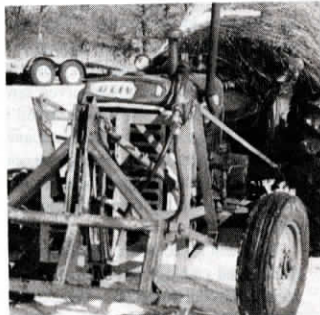
Innovative new front 3-pt. attaches to tractor with a pair of chains.
