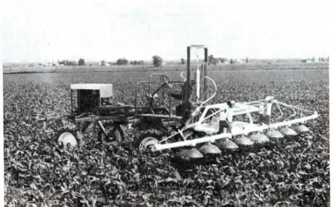
Electric fertilizer machine has eight round plastic hoods positioned about 17 in. above crop. Electricity travels through wires to 1 1/2-in. dia. steel brushes in each hood.
