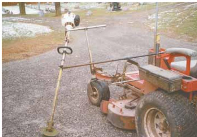
Trimmer hangs from a T-bar mounted just ahead of mower's front wheel.
