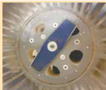
A 12-in. long rotating blade mounts inside the garbage can, direct-driven by an electric motor that bolts on under the platform. Shredded leaves fall through five 3-in. dia. pvc tubes and into the container.
