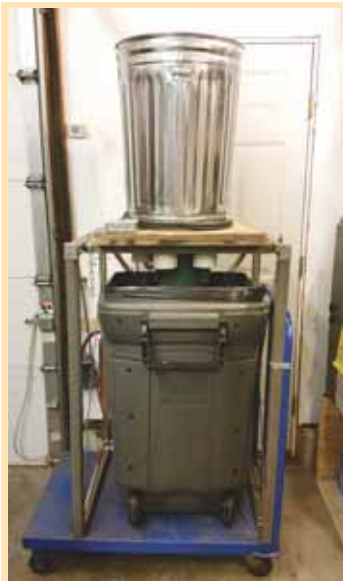
High-volume shredder uses a 20-gal. galvanized metal garbage can, bolted onto a plywood frame above a wheeled trash bin.
