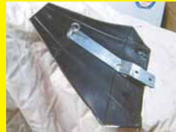
on it that fits into a holding bracket. The problem is that on bumpy roads the strap can easily bounce out of the bracket, and the driver won't even know. A replacement sign costs \$10 or more.
