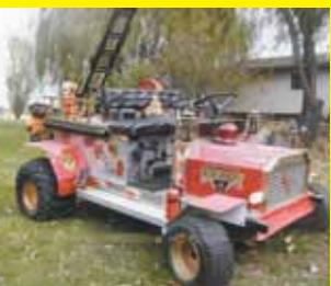
A friend of mine gave me a Kawasaki Mule that had burned up in a garage fire. The only salvageable part was the drive axle so I cut off the frame right ahead of the axle and then started building a miniature fire truck. Kids love it. Comes complete with a ladder, flashing lights, and a siren.
