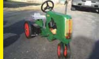
A few years ago FARM SHOW published a story on how I motorized a 1965 Deere Pedal Trac pedal tractor (Vol. 35, No. 3). Since then I've motorized several other brands of pedal tractors, including a pair of Deere 5020's, an Oliver, and a Western Flyer. All are powered by a 1981 Echo 21 cc weed trimmer engine that's hooked up to the transmission off
