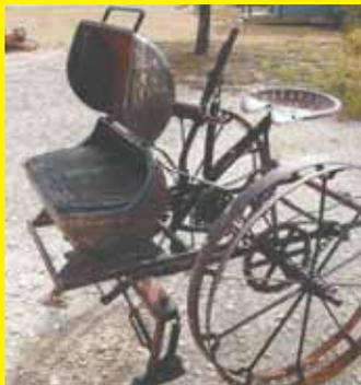
I built a barbeque grill out of an antique seeder with a propane tank mounted on front. I cut the tank open and installed a handle, hinges, and a grill. It looks pretty nifty and we can roll it around to wherever we want to use it. (**Joel Lawler, 282 PR 265, Bowie, Texas 76230 hillbilly265@att.net**)
