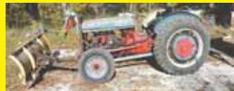
I modified an old Jeep snowplow to mount on my old Ford 9N tractor. I added braces under the tractor from back to front and also added braces on front to hold a hanger that supports a hydraulic cylinder, which is used to raise or lower the blade. The cylinder operates off the tractor's hydraulics. A shut-off valve is used to raise or lower the blade. (**Jerry Brandt, 610 Webster St., La Grange, Mo. 63448 ph 573 655-2260**)
