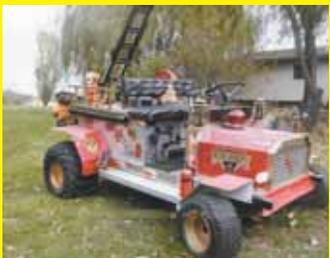
A friend of mine gave me a Kawasaki Mule that had burned up in a garage fire. The only salvageable part was the drive axle so I cut off the frame right ahead of the axle and then started building a miniature fire truck. Kids love it. Comes complete with a ladder, flashing lights, and a siren.
