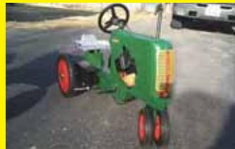
A few years ago FARM SHOW published a story on how I motorized a 1965 Deere Pedal Trac pedal tractor (Vol. 35, No. 3). Since then I've motorized several other brands of pedal tractors, including a pair of Deere 5020's, an Oliver, and a Western Flyer. All are powered by a 1981 Echo 21 cc weed trimmer engine that's hooked up to the transmission off
