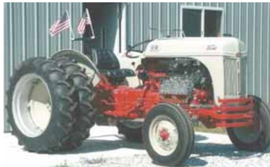
Tom Pike repowered his Ford 8N tractor with a 100 hp, flathead V-8 engine. He also upgraded to a 12-volt electrical system.
