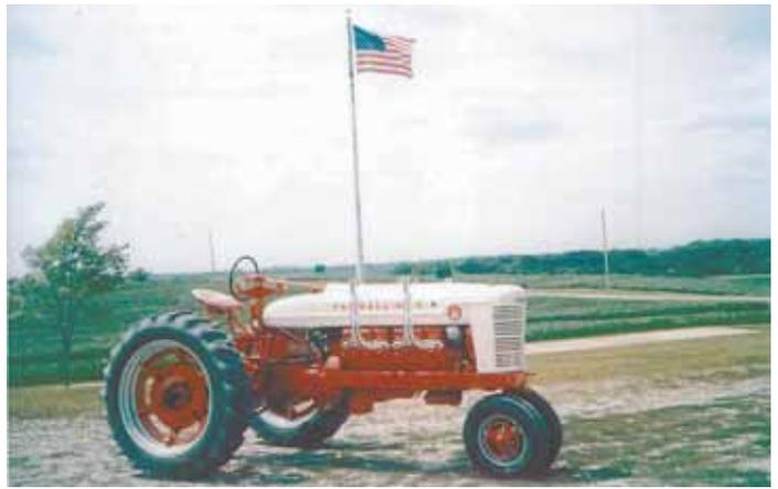
Don Scholting and his son replaced the 4-cyl. gas engine in their 1950 Farmall M with a 275 hp V-12. "We had to stretch the frame 22 in. to fit the bigger engine," he says.
