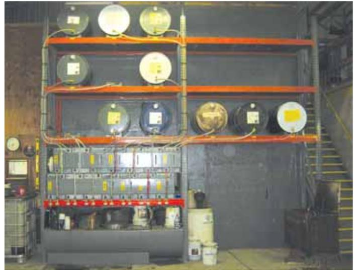
Several 55-gal. drums set on the top 3 racks, while 14 rectangular 30-gal. clear plastic tanks set on the lower 2 racks and serve as reserves. Oil gravity-flows from the drums into the tanks, and from there through hoses fitted with ball valves. A 250-gal. overflow containment tank on the floor catches any spillage.
