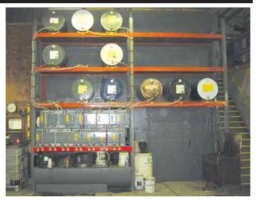
Several 55-gal. drums set on the top 3 racks, while 14 rectangular 30-gal. clear plastic tanks set on the lower 2 racks and serve as reserves. Oil gravity-flows from the drums into the tanks, and from there through hoses fitted with ball valves. A 250-gal. overflow containment tank on the floor catches any spillage.
