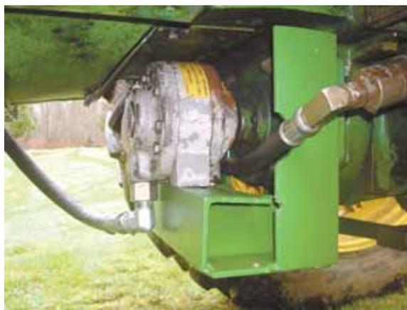
Auxiliary pto-driven hydraulic pump is bolted on front of the transmission on Larry McPhail's Deere 4010 tractor.
