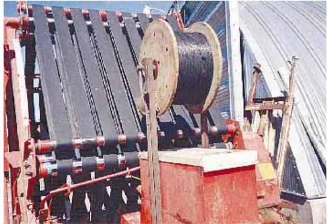
Falkowski ties old twine together end-to-end and winds it up on empty 2-ft. dia. wooden welding wire spools. Twine feeds into baler just like it would out of twine box.
