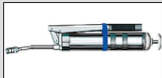
my grease gun to keep the handle closed. How many times do you pick up your gun and the handle is cocked. When you close it, you lose a shot of grease. I just slide the wrist band up over the handle and tube body. Saves grease and holds your gun neatly."
