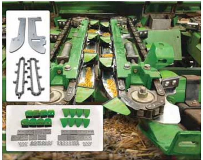
"Operation Harvest Sweep" system replaces existing deck plates and gathering chains on corn headers with components designed to reduce shatter loss.
