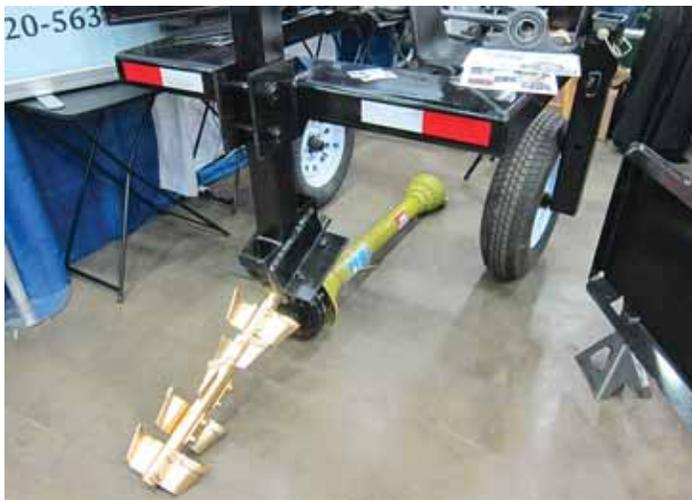
Twister Trencher consists of a pto-driven hardened shaft fitted with a series of cutting blades that penetrate dry, hard-packed soil.
