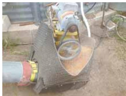
AugerBox is designed to enclose a discharge auger and funnel any flying grain down into the transport auger, minimizing waste and clean up.
