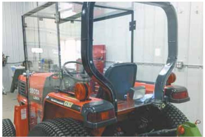
Blackburn bought the plexiglass in 4 by 8 sheets and cut everything to fit. He used 1-in. steel tubing to make a 4-section frame and attached the back piece to the rollbar.
