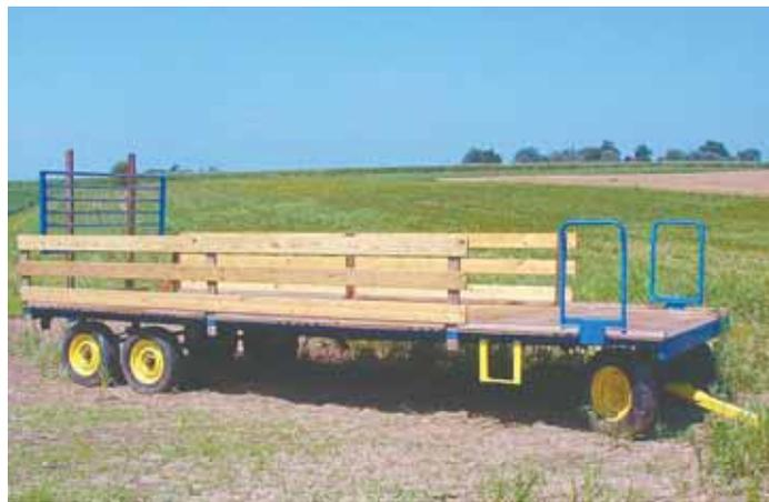
At 21 ft. long, the triple axle wagon is about 4 ft. longer and 1 ft. wider than most hay wagons and can load about 25 more bales.
