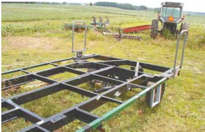
Wagon has angle iron ladder steps and front handholds on both sides, allowing the person stacking bales to stand safely at front of wagon as it lurches across the field.
