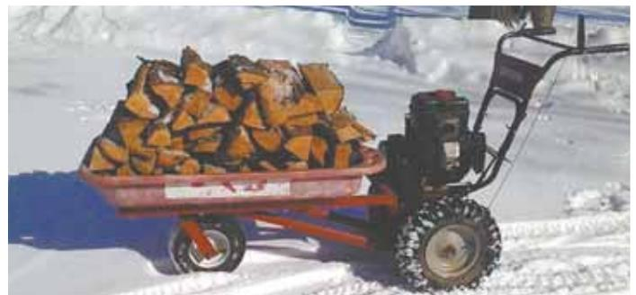
**Bledsoe unbolted the blower and auger from a walk-behind snowblower and mounted a small wagon box in their place. It rides on a single caster wheel.**
