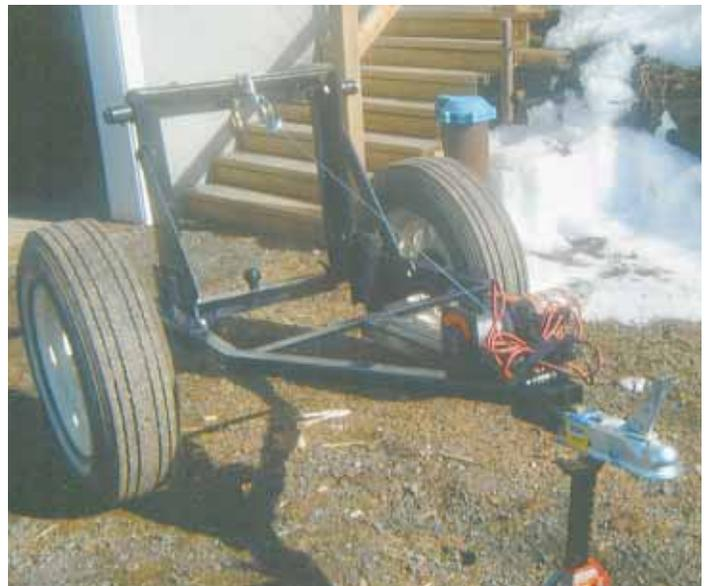
**Phil Harris uses his power winch-equipped log hauler to pick up the end of a log. A removable crossbar on back with a ball hitch can be used to tow a trailer.**
