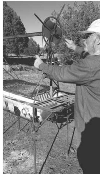
Baughman cut a rectangular opening in the bottom of the tub and installed a metal plate over the opening, attached to a rod that runs the length of the tub and has a horseshoe fastened to one end of it. When he turns the horseshoe, the bar rotates the plate and the ashes fall out.
