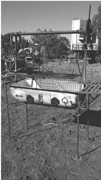
Bathtub sets up about 2 ft. off the ground. The 4-ft. long open grill inside it can be easily raised and lowered by turning a big wheel located at one end of the tub.
