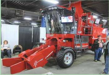
Self-propelled, 4-WD Bale Baron eliminates the need for a tractor to make tightly bound blocks of up to 21 bales.
