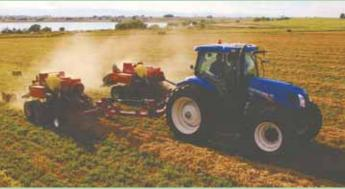
PowerLinx dual power hitch lets you operate 2 small square balers at once. It takes the pto power from one tractor and splits it in two.
