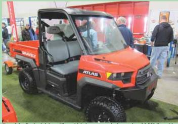
Gravely's all-wheel-drive utility vehicle has a cargo bed capacity of 1,250 lbs. with a
