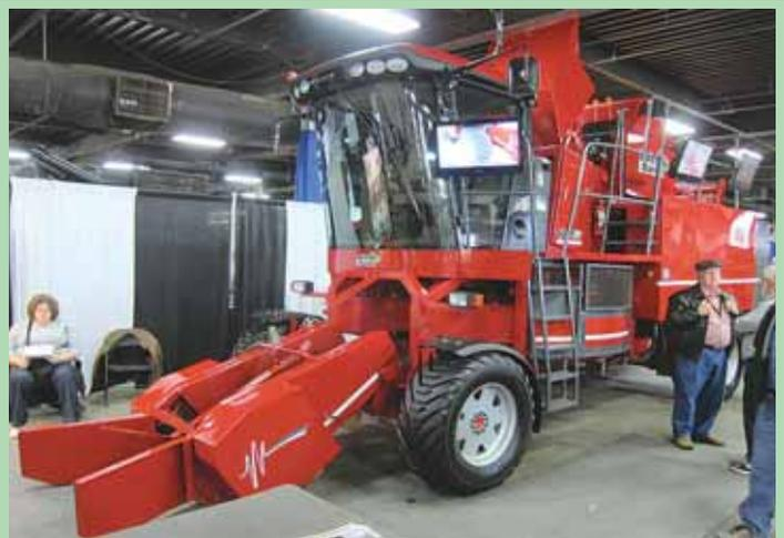
Self-propelled, 4-WD Bale Baron eliminates the need for a tractor to make tightly bound blocks of up to 21 bales.
