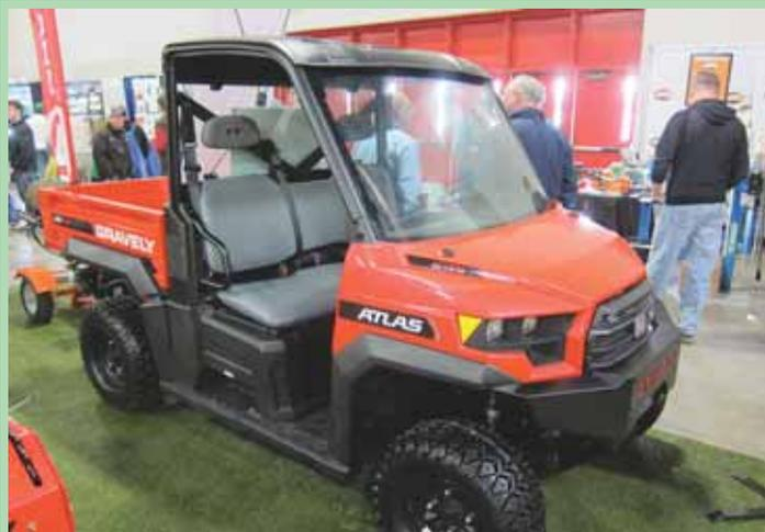
Gravelly's all-wheel-drive utility vehicle has a cargo bed capacity of 1,250 lbs. with a full ton of towing capacity.
