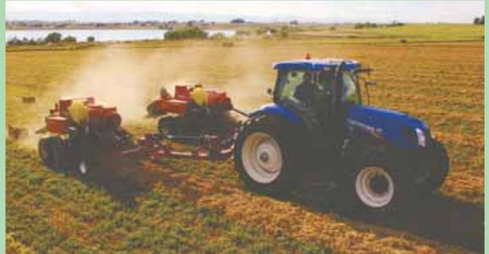
PowerLinx dual power hitch lets you operate 2 small square balers at once. It takes the pto power from one tractor and splits it in two.
