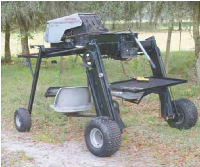
Paul King built this 2-man, self-propelled harvesting cart out of a Craftsman riding mower. Cart still has the mower's original engine, transmission, rear axle and wheels.
