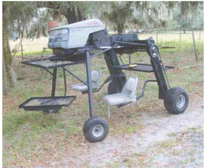
Engine and drivetrain mount 4 ft. off the ground, above operators. Both rear wheels are belt-driven.
