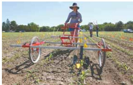
Weed Master's parallel linkage design makes it easy to use a variety of tillage tools, such as this hiller attachment.
