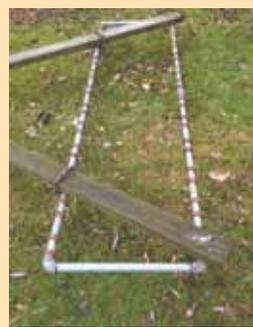
Roland Erikson pulls this 74-in. wide rake behind his riding mower to remove debris from his yard. Rake's 24 tines attach to 2 galvanized water pipes.
