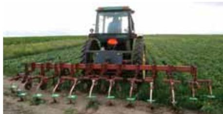
This 12-row, 20-in. Case IH VibraShank cultivator is fitted with Profit Organics' Flow Shields.
