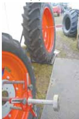
System uses a laser attached to the wheel rim to make sure big tractor tires are aligned, reducing wear and lowering fuel consumption.
