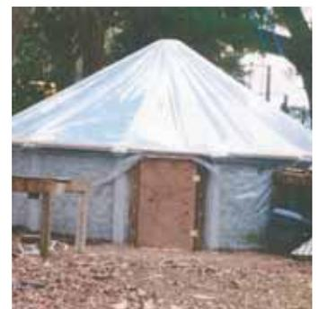
Robert Witt converted an 18-ft. dia. by 3-ft. high above-ground swimming pool into a low-cost greenhouse, building a roof and covering it with clear greenhouse film.
